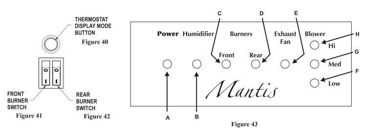
**Caution:** When switching from the front burner to the rear burner, be sure to activate the rear burner first, then turn off the front burner. When switching from rear burner to the front burner, be sure to activate the front burner first. Simple rule - always activate the desired burner first, then switch the other burner off. If it is switched the wrong way, the burner(s) will go out and the heater may need to be reset. Refer to page 47 - Resetting the Heater.
